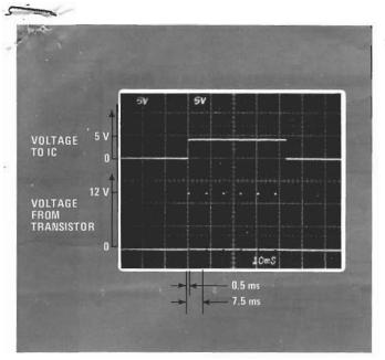
**2. Pulses to ignition.** Upper trace shows voltage waveform at B input of mono A due to points opening. Lower trace shows the resulting train of pulses, which triggers the solid-state ignition six times. The train of pulses is terminated when the points close.
